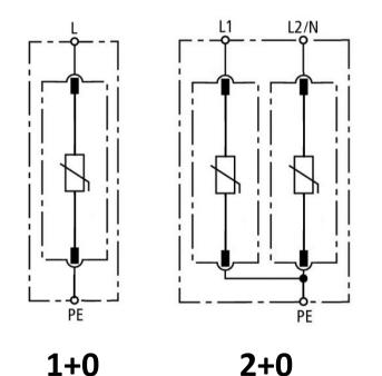
Phase to PE via Metal oxide Varistor (MOV) With each device in its own Cartridge
